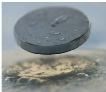
A magnet floats on the magnetic field of a superconductive material, the precursor state of the appropriately named strange metals.
